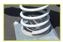
**3- The spring** is made from Grade 35SCD6 steel, shot blasted, stress relieved, zinc coated and finished with two coats of epoxy polyester powder.
