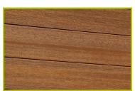
2- The blades are made of wood-plastic composites (WPCs), 95% of which is recycled plastic material (HDPE) and post-industrial wood sawdust. They are covered with a thin decorative brown wooden layer, which makes the material resistant and waterproof, and ensures the colours do not alter over time. The planks do not require specific maintenance.
