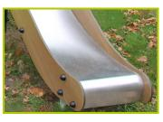
**7- The sliding surface** is made of 2mm thick stainless steel, which is shaped, bent and rolled from one piece.
