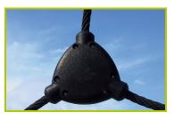
**7- The 16mm diameter rope** is made of galvanised steel cable covered with polyester. The net fittings are made of polyamide and used to link three cords together.
