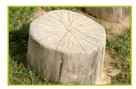
2- The stair treads (with average diameter 25 to 30cm) are made from sap free robinia. The robinia is sanded and has had its bark removed. Robinia is naturally rot proof and does not require any additional chemical protection; it is equally extremely resistant to attacks from external sources (insects, fungi, climatic variations), guaranteeing the long term durability of the playground equipment.
