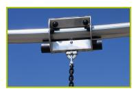
**3- The one-piece rail** is made of stainless steel, Ø 76.1mm, 3.6mm thick. The trolley is made of stainless steel ensuring its durability.
