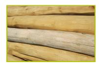
1- The different posts (average diameter: 100 to 120mm / 120 to 140mm) are made from sap free robinia. The robinia is sanded and has had its bark removed. Robinia is naturally rot proof and does not require any additional chemical protection; it is equally extremely resistant to attacks from external sources (insects, fungi, climatic variations), guaranteeing the long term durability of the playground equipment.
