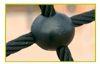
**2- The 16mm diameter ropes** are made of galvanised steel cable covered with polyester. The cables are linked together and held in place by injected polyamide spheres.
