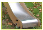
**6- The sliding surface** is made of 2mm thick stainless steel, which is shaped, bent and rolled from one piece.
