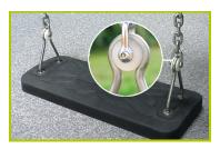
**11-The swing seats** are made of shock absorbing moulded honeycomb rubber. The swing chains are made of galvanised steel. The seat fixing brackets are made of 10mm stainless steel wire. PVC sliding rings are fitted to limit the wear of the metal parts over time. The rings are accessed by a vandal proof, stainless steel shackle.
