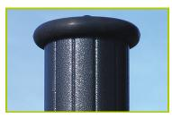
2- The 125mm diameter post is made of painted galvanised steel. The two-tone grey grained finish has a slightly undulating surface for increased scratch resistance. The cap is made of injection moulded polyamide.
