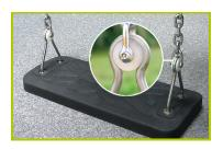
**11-The swing seats** are made of shock absorbing moulded honeycomb rubber. The swing chains are made of galvanised steel. The seat fixing brackets are made of 10mm stainless steel wire. PVC sliding rings are fitted to limit the wear of the metal parts over time. The rings are accessed by a vandal proof, stainless steel shackle.
