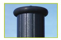
**2- The 125mm diameter post** is made of painted galvanised steel. The two-tone grey grained finish has a slightly undulating surface for increased scratch resistance. The cap is made of injection moulded polyamide.
