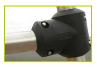
**7- Injection moulded polyamide fixings** connect the posts with the platforms and the various play features. They are non-toxic, flameproof and U.V. resistant. The thickness of the polyamide makes the equipment both strong and vandal resistant.
