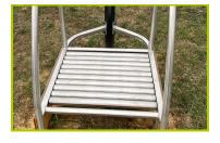
**18-The Runner rolling bars and surrounding frame structure** are made of stainless steel.
