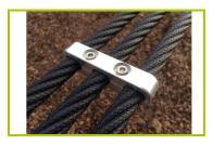
**7- The strap** is made of 3 ropes linked together with aluminium pliers. Each rope, of 16mm diameter, is made up of galvanized steel cables covered in polypropylene.
