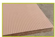
**3- The platforms** are made from a 12.5mm thick, textured, non-slip compact material (HPL).
